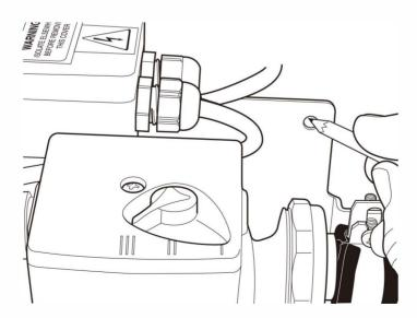
Remove the unit and drill (8mm masonry drill) and plug the holes. Align and secure the unit to the wall with the screws provided. The unit is now ready for connecting to the primary heating supply and underfloor heating loops. If appropriate the unit can be connected to the underfloor heating loop(s), filled and pressurised via the integral ball valves and then locked off for floor screeding before making the boiler connection.
